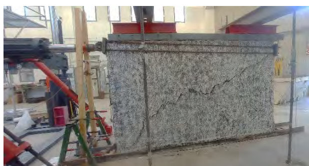
Laboratory test on brickwork reinforced with TRM
