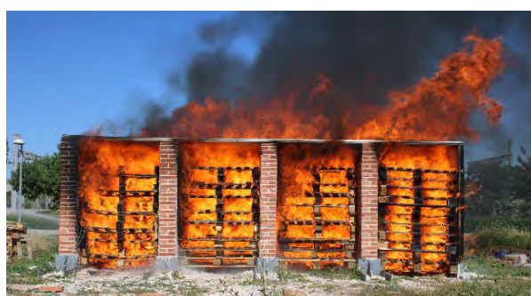
Test on several brick masonries reinforced with TRM on one or both faces
