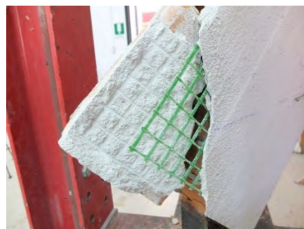
Fig. 2: Shear Strengthening of Masonry
