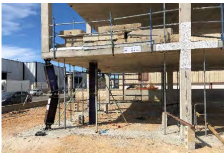
Testing a full-scale building subjected to column-removal scenarios
