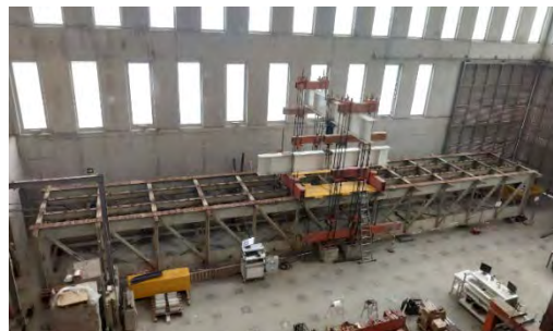
Testing a real steel riveted railway bridge (built in 1915) to analyse its robustness after failing some of its elements
