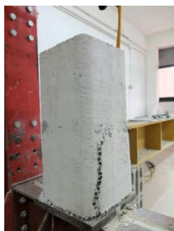
Fig. 1: Confinement of Masonry Columns
